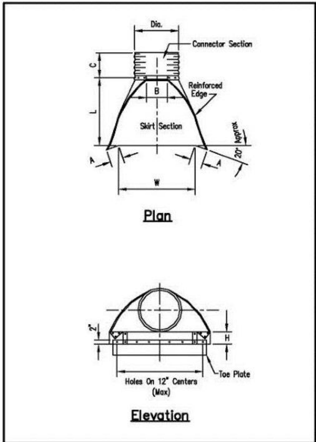
Figure TSD-2 Flared End-Section Detail
