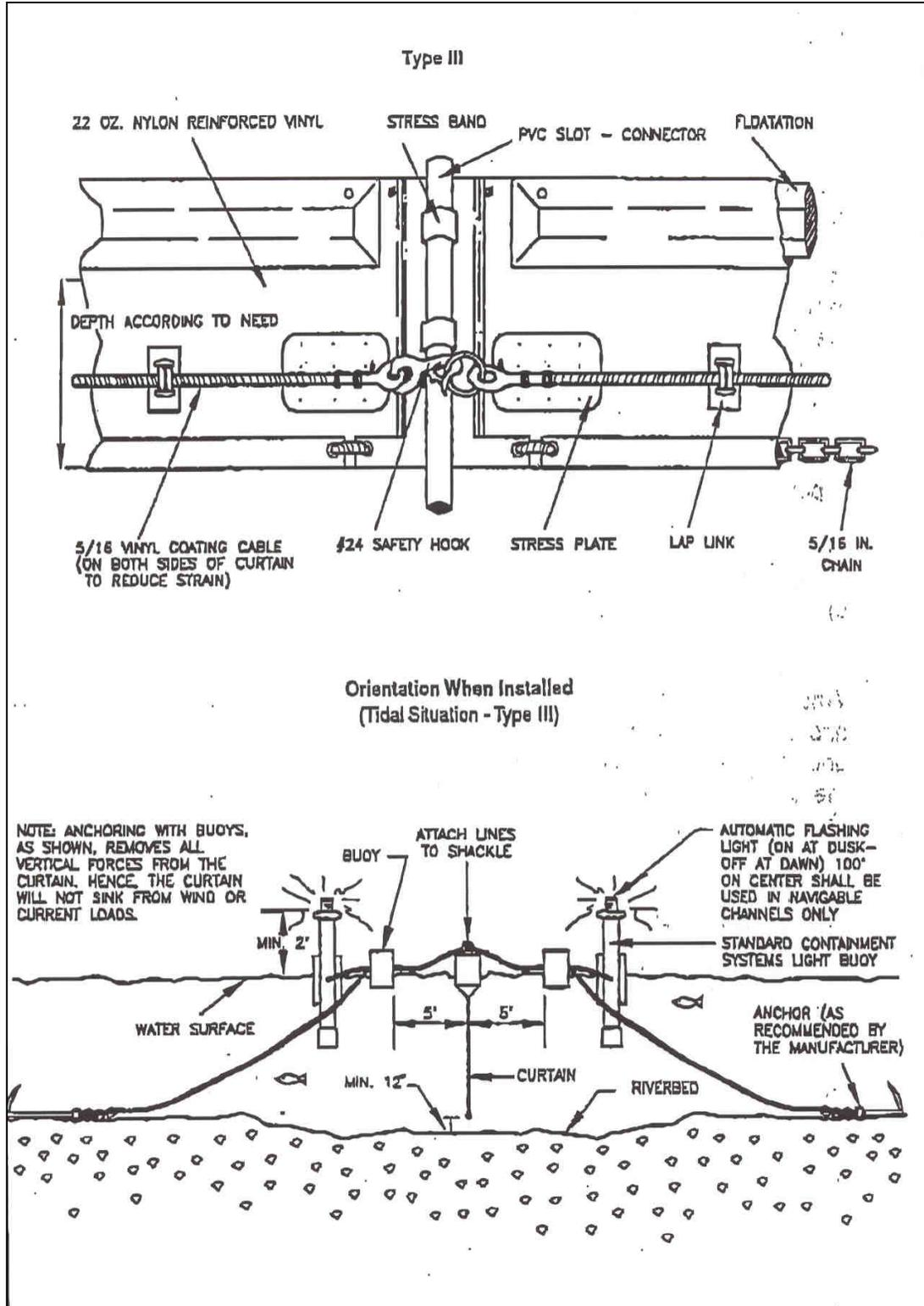
Figure FB-2 Type III Floating Turbidity Barrier
