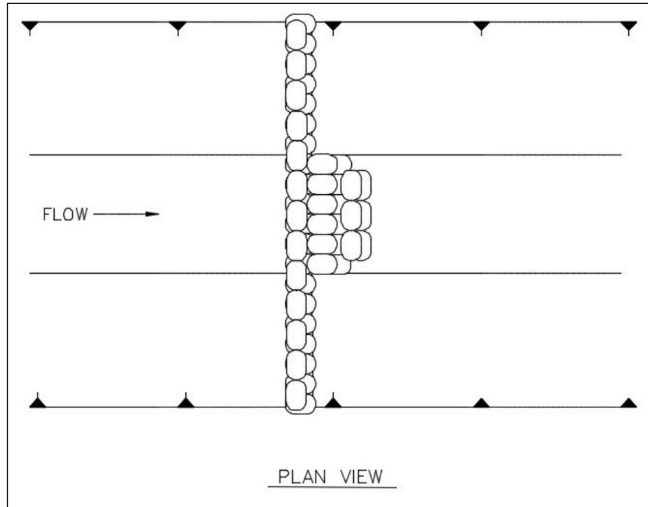
Figure CD-9 Sand Bag Check Dam Plan View
