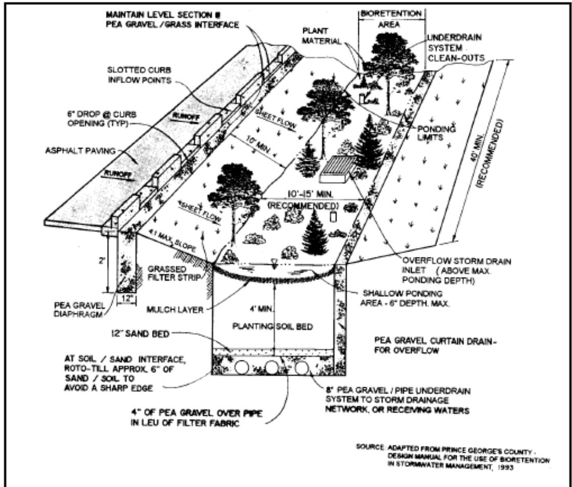
Figure BA-2 Typical Bioretention Area
