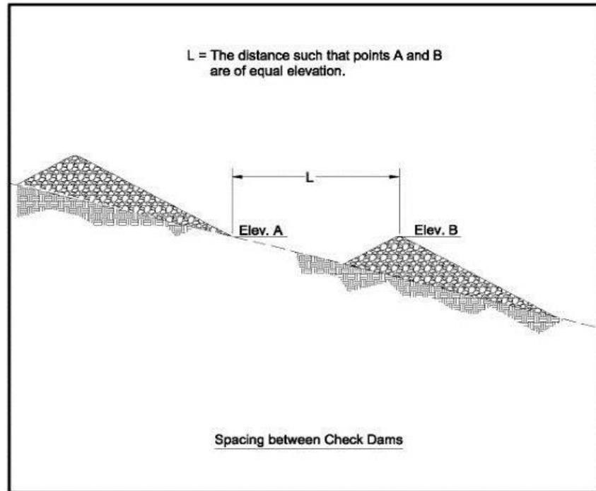
Figure CD-2 Profile of Typical Rock Check Dams
