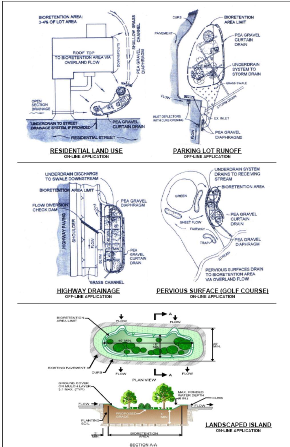
Figure BA-1 Applications of Bioretention Areas
