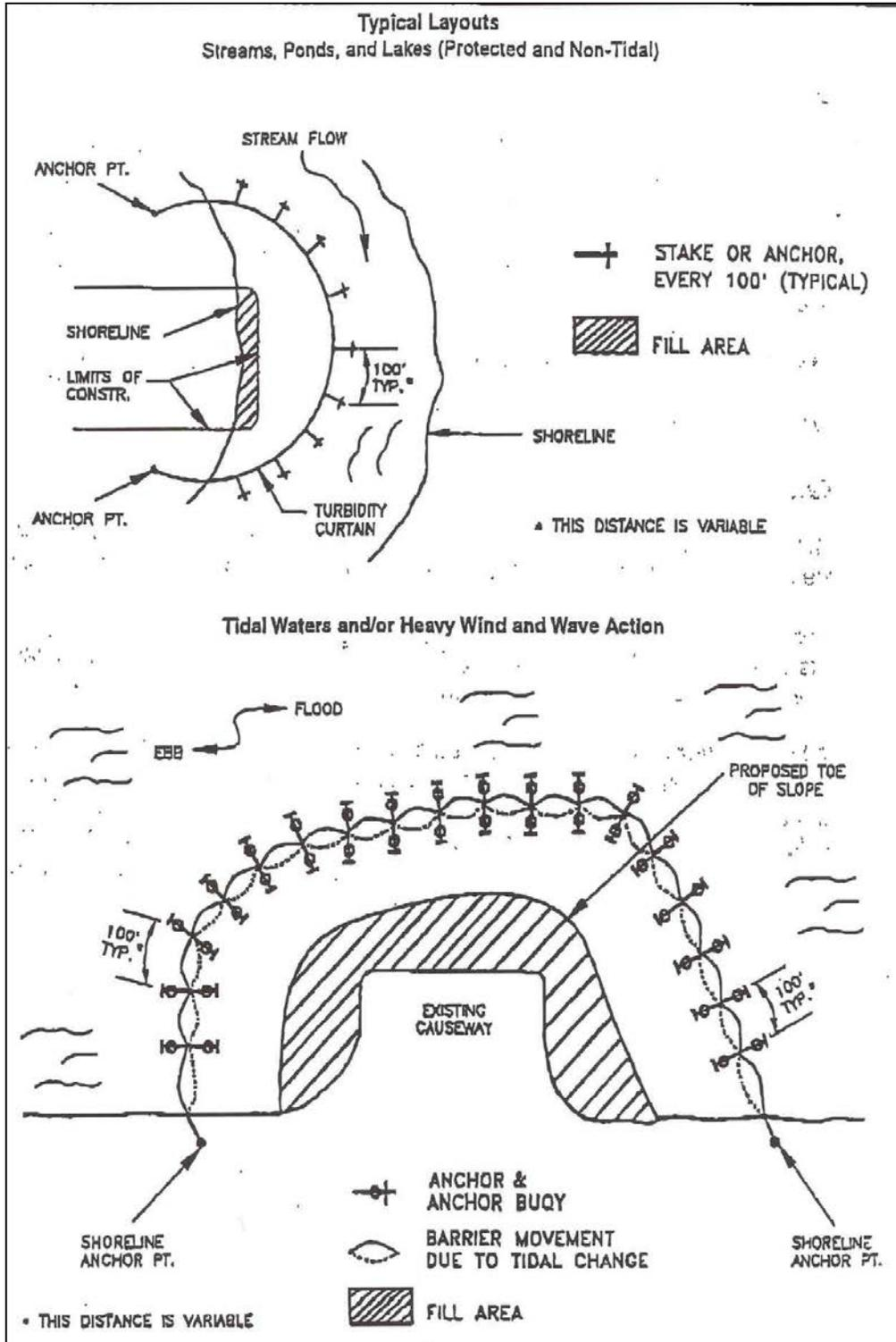
Figure FB-3 Typical Installation Layouts
