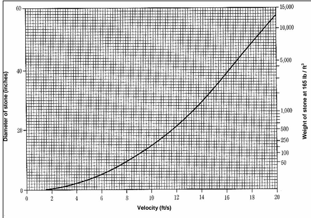
Figure CS-1 Ishbash Curve
