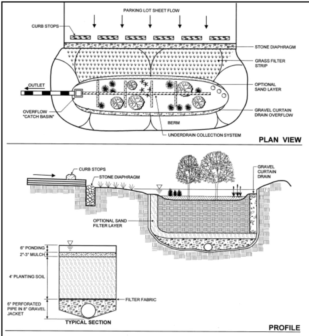
Figure BA-3 Typical On-line Bioretention Facility
