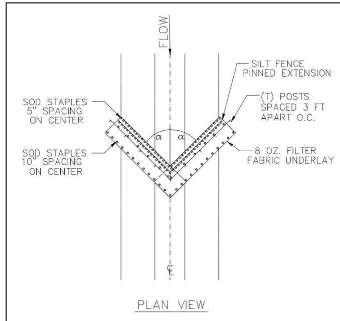
Figure CD-6 Silt Fence Check Dam Plan View
