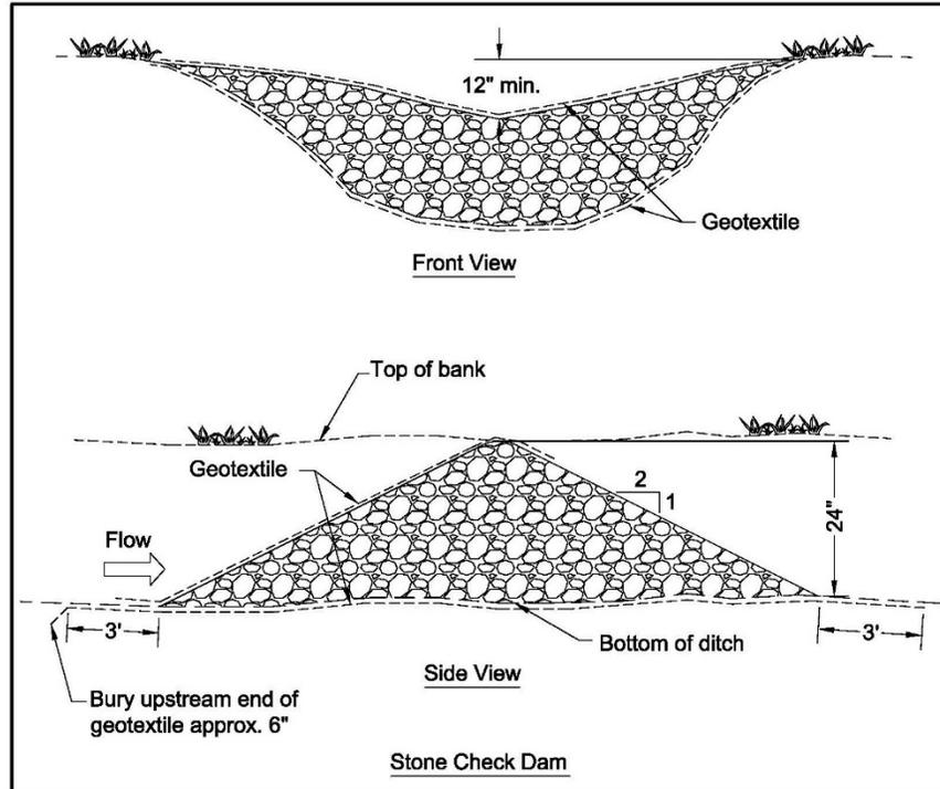
Figure CD-1 Profile and Cross-Section of Typical Rock Check Dams
