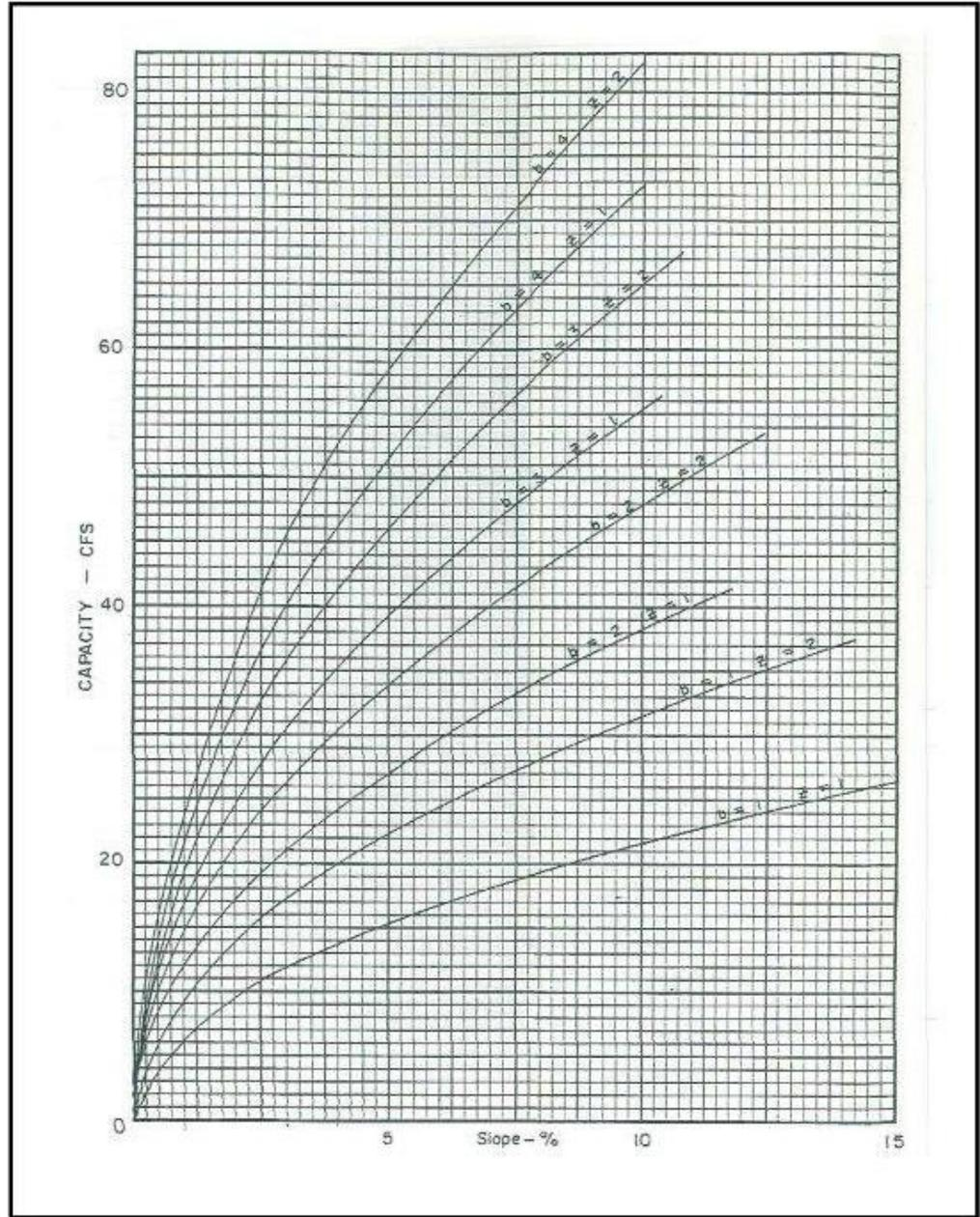
Figure LS-2 Capacity Graph for Concrete Flumes
