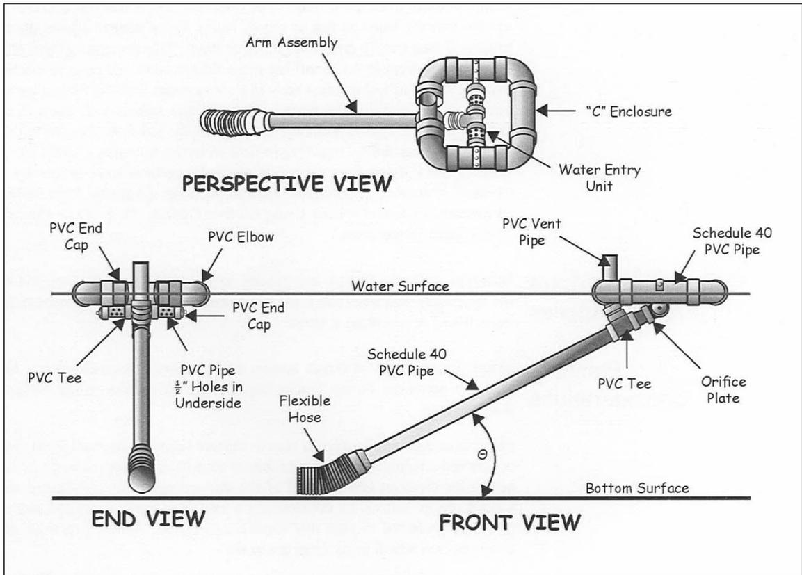
Figure SBN-4: Schematic of a skimmer
