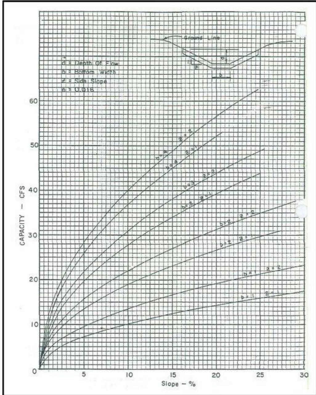
Figure LS-1 Capacity Graph for Concrete Flumes
