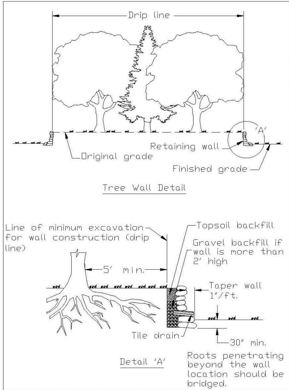
Figure PV-4 Tree Wall Detail
