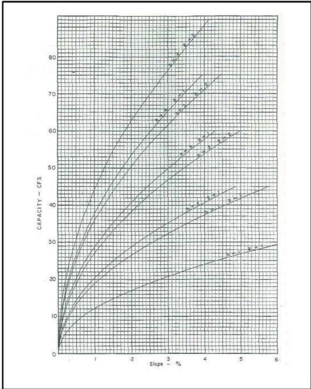
Figure LS-3 Capacity Graph for Concrete Flumes
