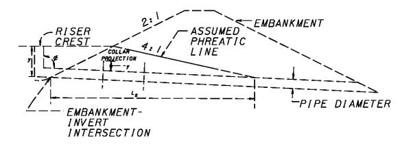
FIGURE 3-12: Anti-Seep Collar Schematic
