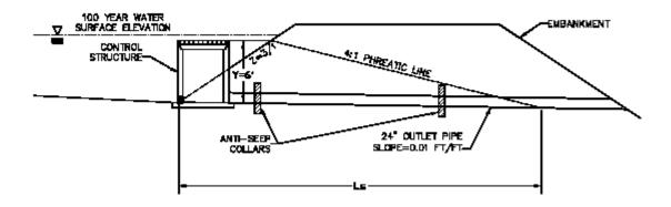
FIGURE 3-13: Anti-Seep Collar Design (Example)
