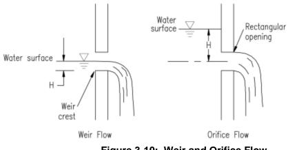
Figure 3-10: Weir and Orifice Flow
