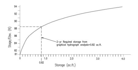
FIGURE 3-8: Stage vs. Storage Curve, Example
