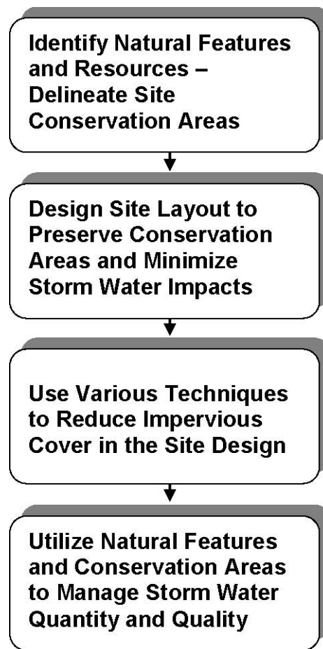
Figure 1.3.1-1 Stormwater Site Design Process
