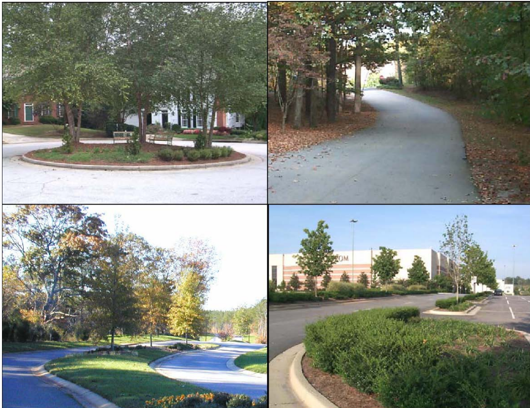
Figure 1.3.2-17 Example of Reducing Impervious Cover (clockwise from upper left): (a) Cul-de-sac with Landscaped Island; (b) Narrower Residential Street; (c) “Green” Parking Lot with Landscaped Islands; and (d) Landscape Median in Roadway.
