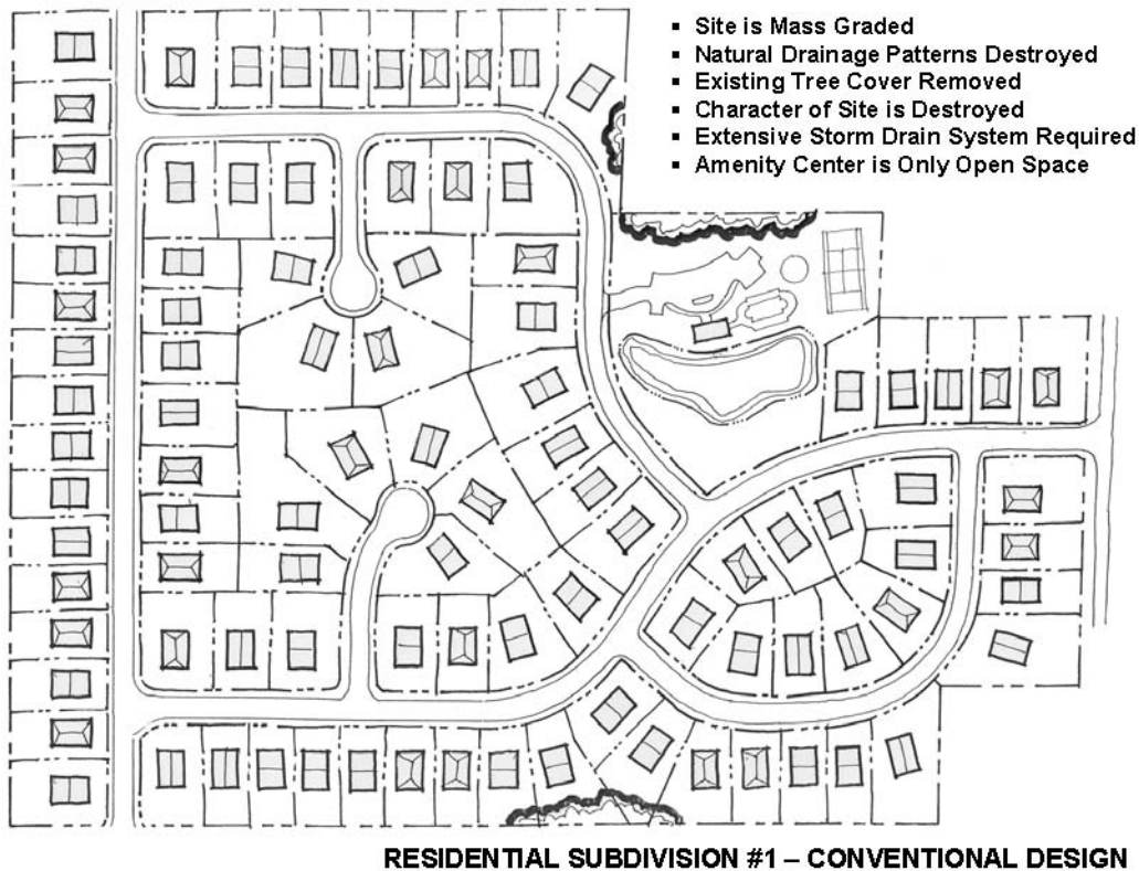
Figure 1.3.3-1 Comparison of a Traditional Residential Subdivision Design (above) with an Innovative Site Plan Developed Using Stormwater Site Design Practices (below).
