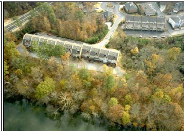
Figure 1.3.2-14 Example of Site Footprinting
