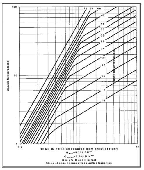
Figure 7-5 – Flow Rates vs. Head (riser)
