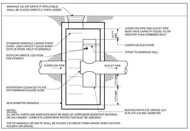
**Figure 7-6 – Flow Control Structure Example**
