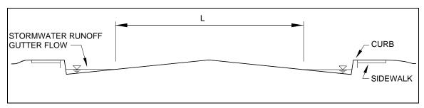
Figure 8-2 – Non-Flooded Road Width (L)
