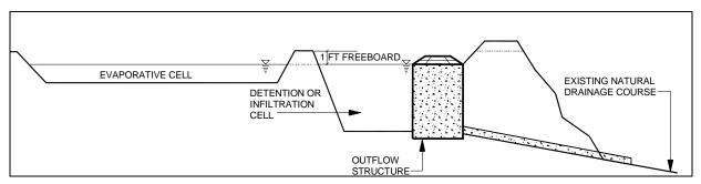
Figure 7-7 – Separated Evaporative/Detention Facility Cross-Section
