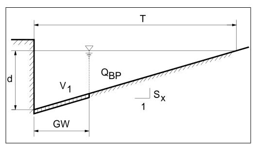
**Figure 8-5 – Typical Grate Inlet Cross-Section**
