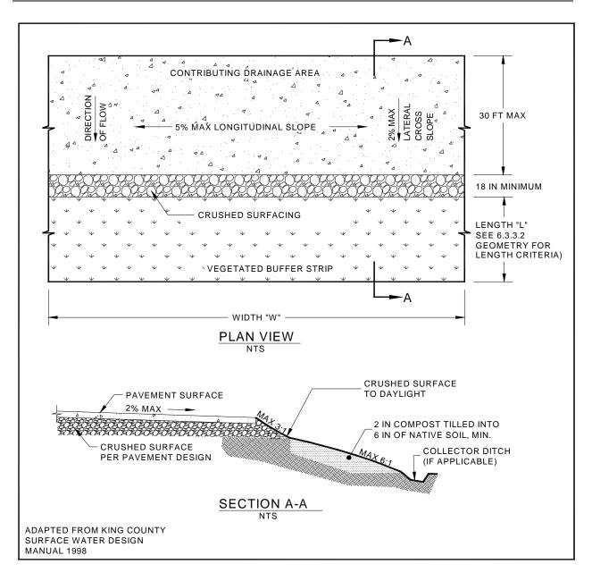
Figure 6-4 – Typical Vegetated Buffer Strip (details)
