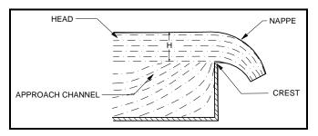
Figure 7-4 – Sharp-Crested Weir
