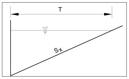
**Figure 8-3** – Uniform Gutter Section
