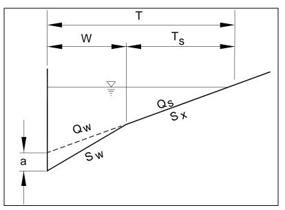
**Figure 8-4 – Composite Gutter Section**
