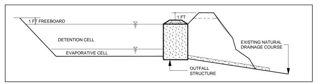
Figure 7-8 – Stacked Evaporative/Detention System Cross-Section
