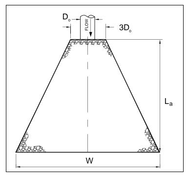
Figure 8-1 – Riprap Revetment at Outfall Schematic
