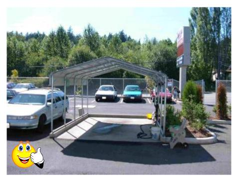
**Figure IC-4b**. The photograph above demonstrates good storm water management practices. A dedicated car wash area at a vehicle repair facility is covered, bermed and graded to drain through an approved pre-treatment device connected to the sanitary sewer. (Source: U.S. EPA)
