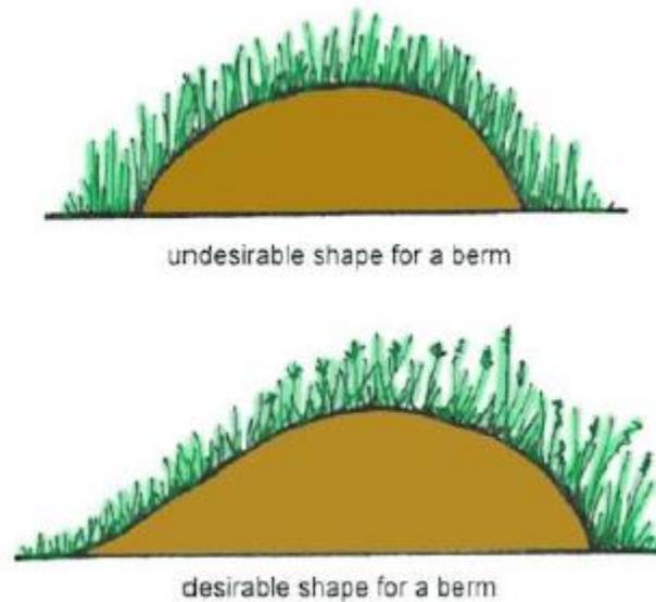
Figure 6-2. Infiltration Berm Shape, Design Guidance
