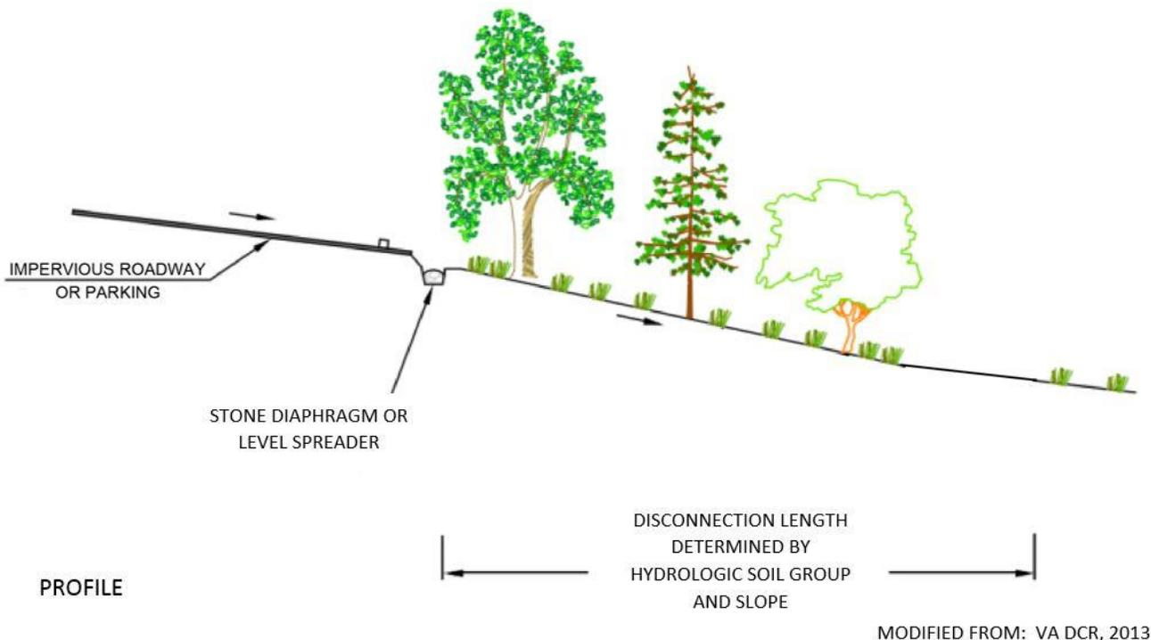
Figure 4-6. Disconnection to Filter Strips and Vegetated Buffers, Design Guidance
