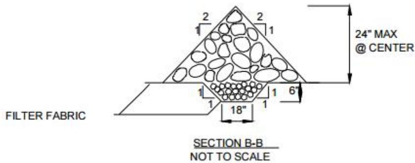
Figure 6-11. Check Dam (Detail), Design Guidance
