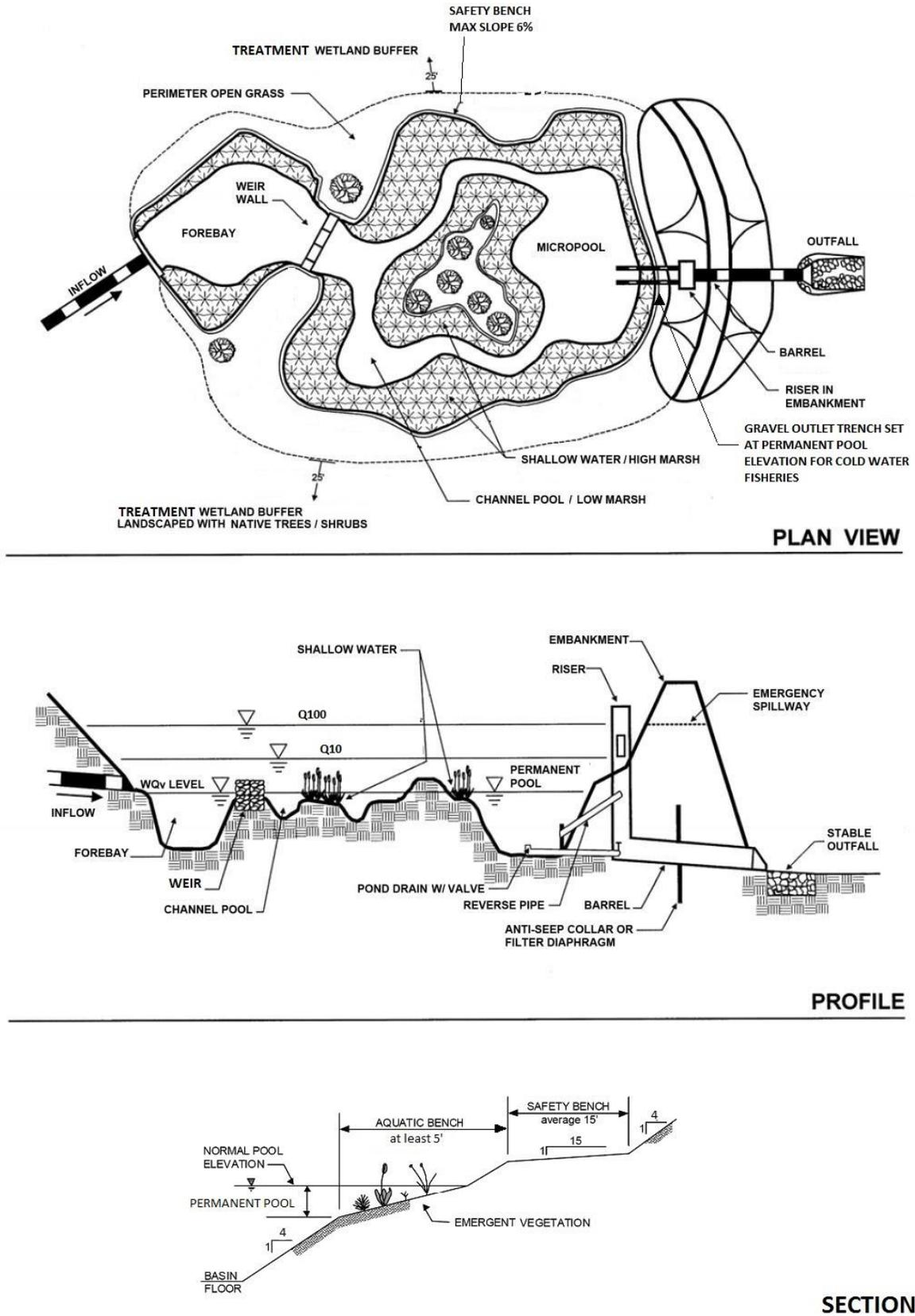
Figure 4-18. Shallow Surface Wetland, Design Guidance
