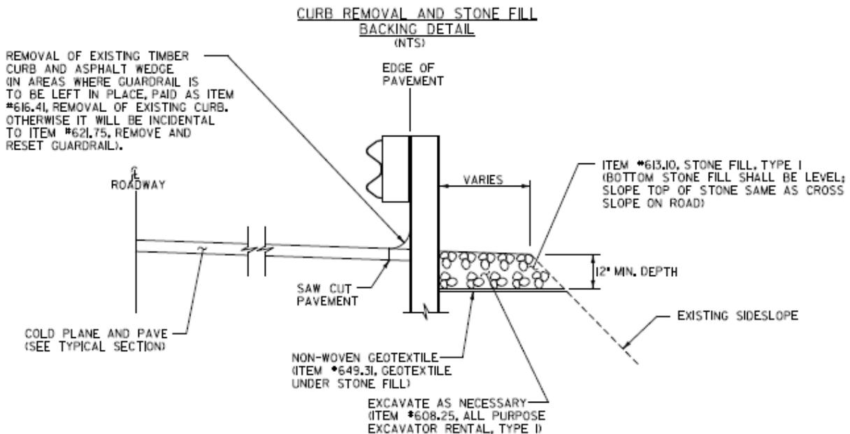
Figure 6-1. Curb Removal (Detail), Design Guidance
