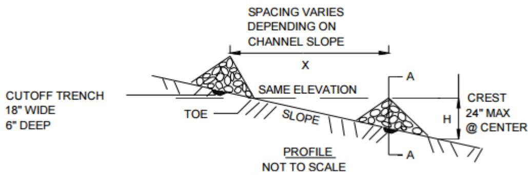
Figure 6-10. Check Dam (Profile), Design Guidance
