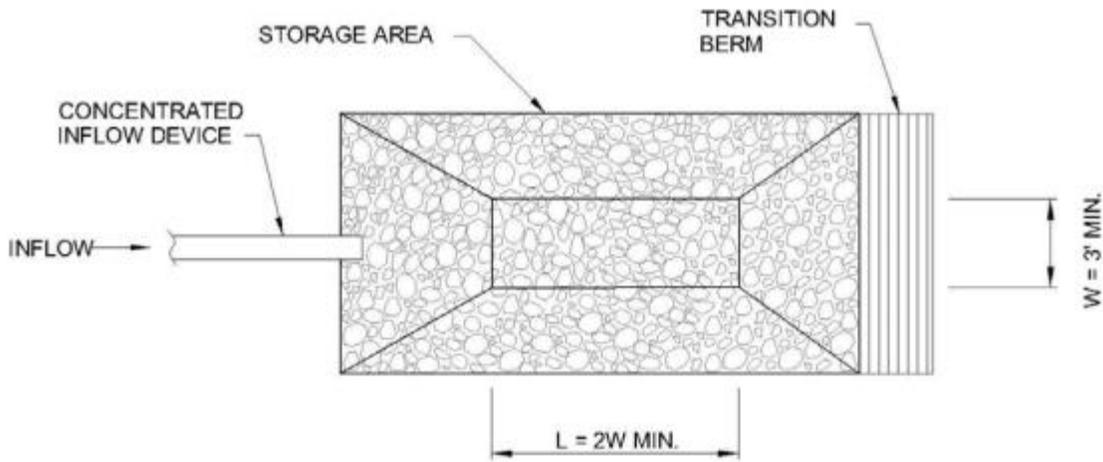
Figure 6-8. Plunge Pool, Rectangular (Plan View) Design Guidance (Source: NCDOT 2014)
