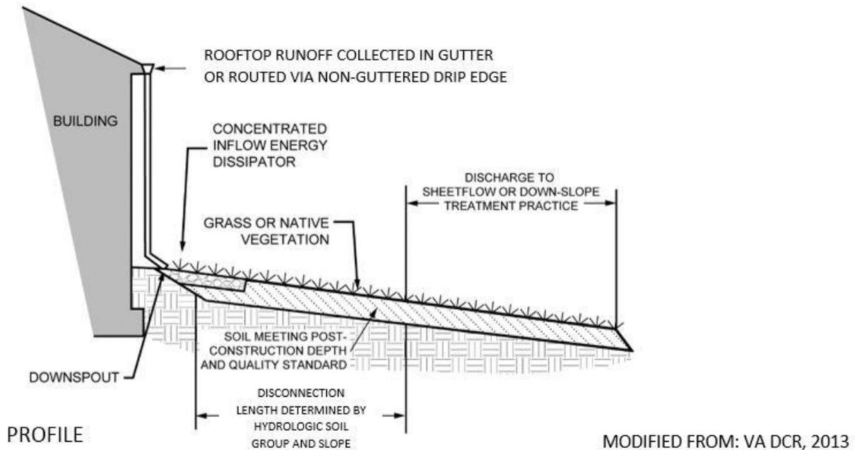
Figure 4-5. Simple Disconnection, Design Guidance
