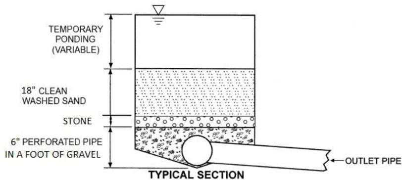
Figure 4-16. Underground Sand Filter, Design Guidance
