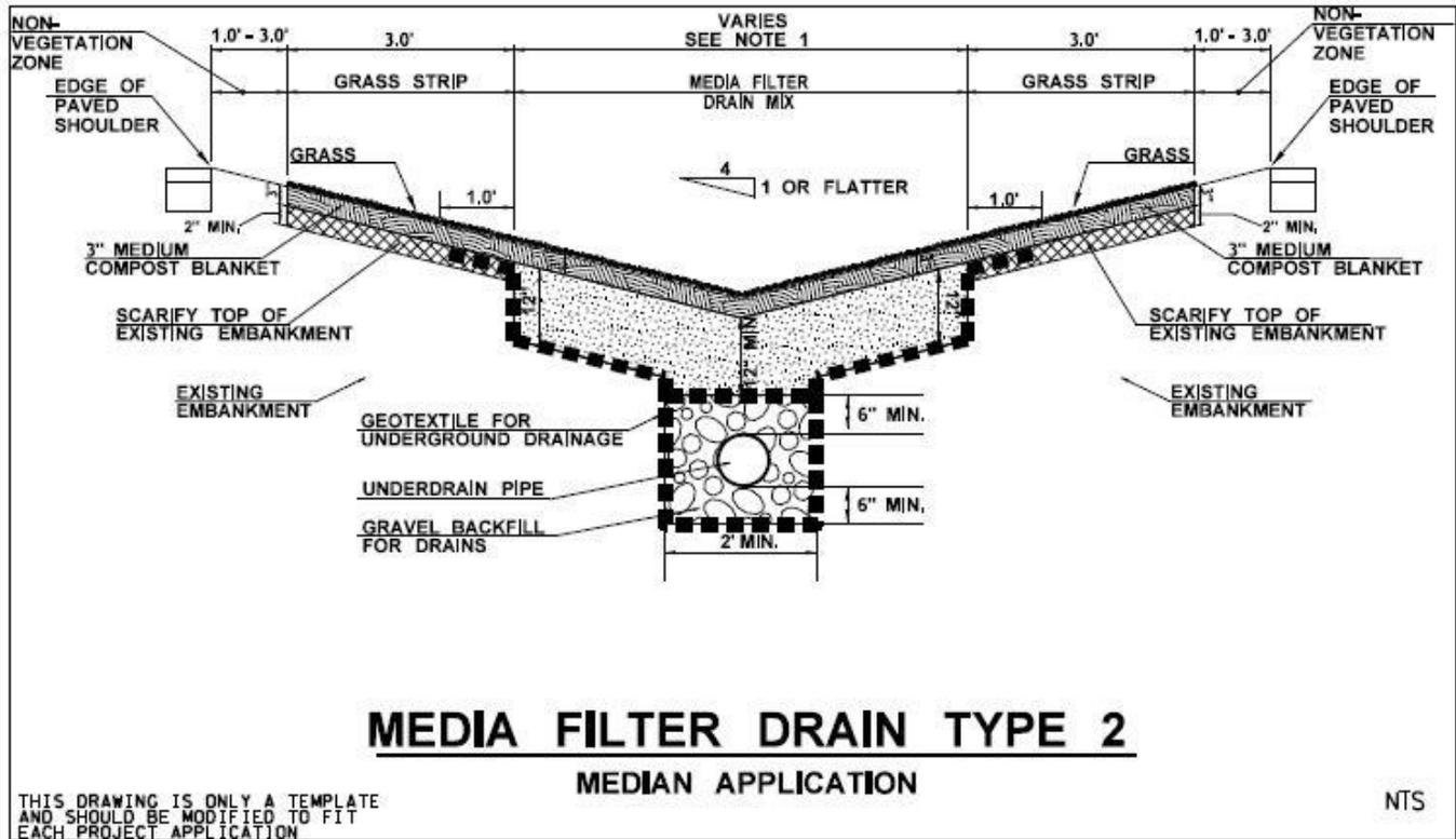
Figure 6-4. Media Filter Drain, Type 2, Design Guidance
