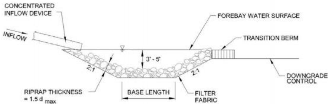
Figure 6-9. Plunge Pool, Rectangular (Profile View), Design Guidance (Source: NCDOT 2014)
