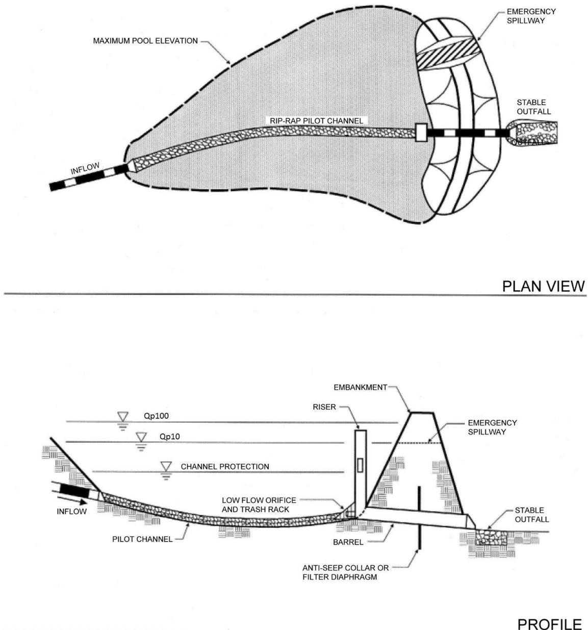
Figure 5-1. Dry Detention Pond, Design Guidance
