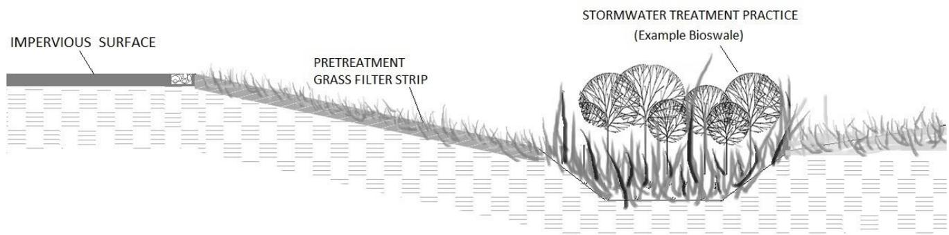
Figure 4-2. Pre-Treatment Filter Strip, Design Guidance
