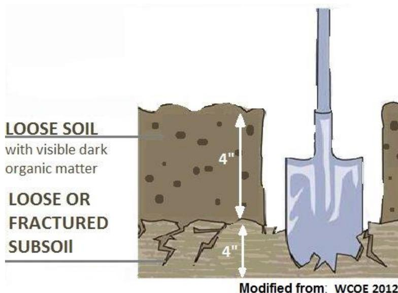
Figure 3-1. Post-Construction Soil Depth and Quality Standard Field Verification, Design Guidance
