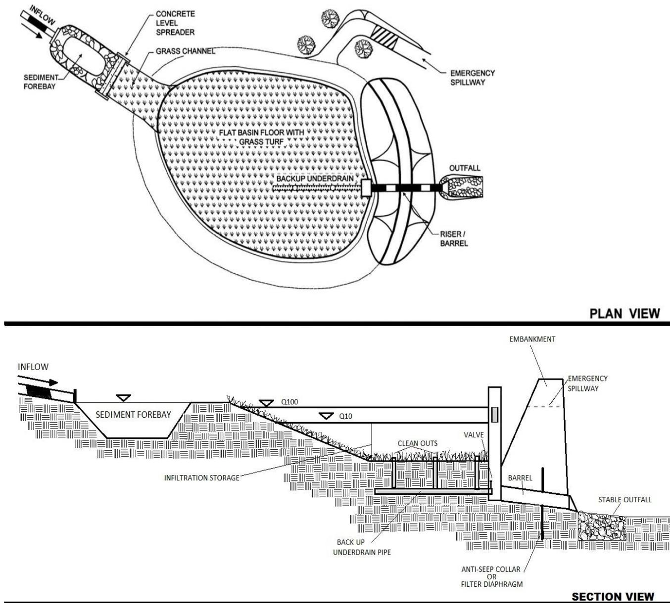
Figure 4-13. Infiltration Basin, Design Guidance
