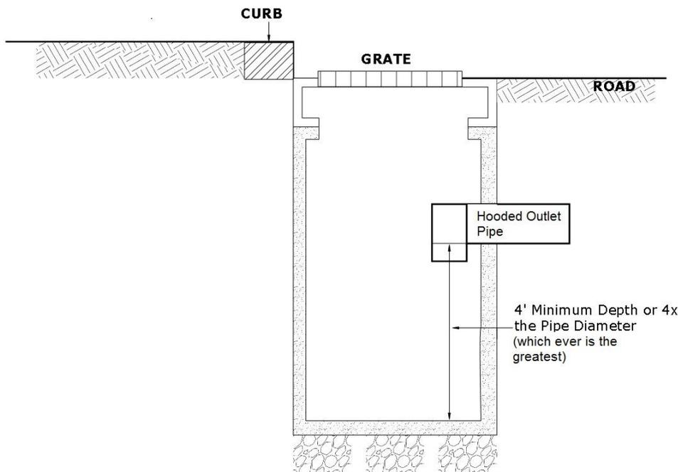
Figure 4-4. Deep Sump Catch Basin, Design Guidance
