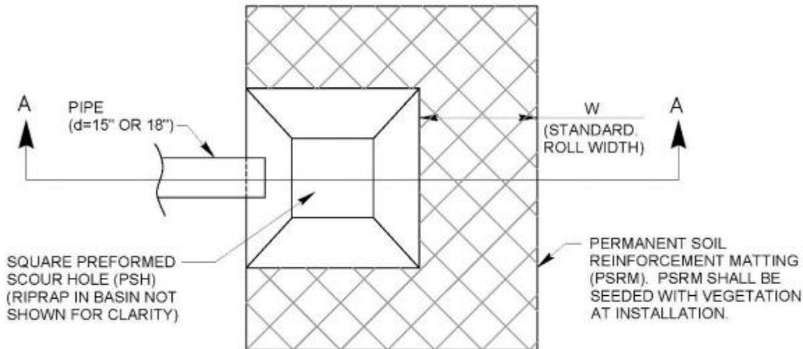
Figure 6-6. Plunge Pool (Plan), Design Guidance (Source: NCDOT 2014)
