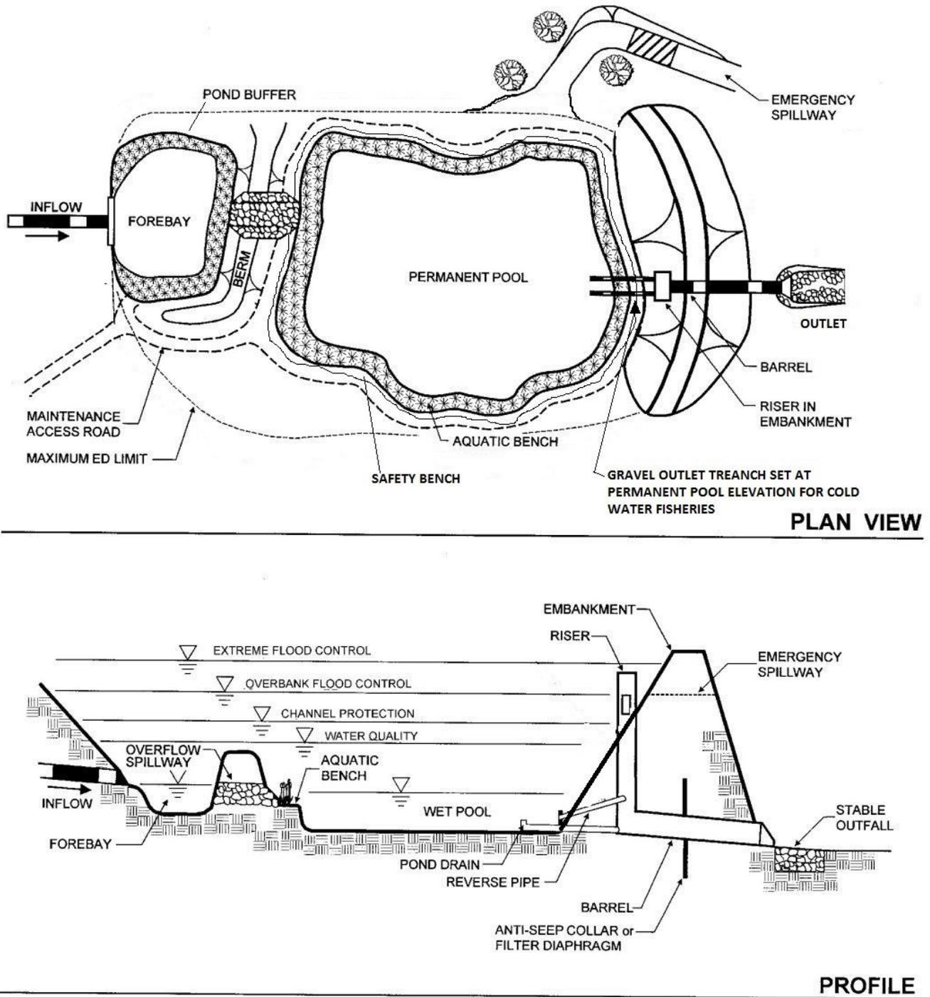
Figure 4-20. Wet Pond, Design Guidance
