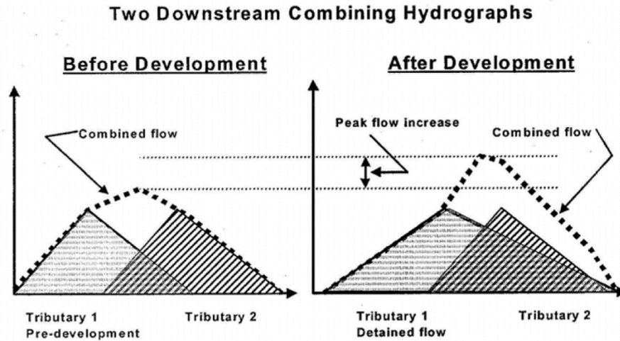
Figure 2-2: Graphical Depiction of Coincident Peak Phenomena (ARC, 2001), Design Guidance
