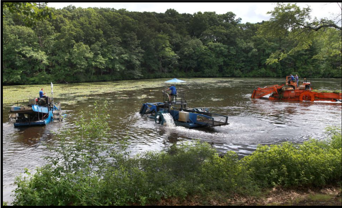
The state had crews using mechanical harvesters to uproot invasive water chestnuts from the Charles River in Waltham .(Photos by Wendy Maeda/Globe Staff)
