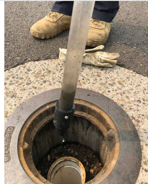
Figure 2: Proprietary device inspection utilizing Sludge Judge monitoring tool for sediment assessment on an Oldcastle isolator row
