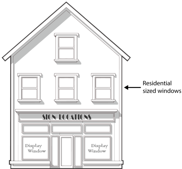
Figure 1333.29E: Building Scale and Proportion
