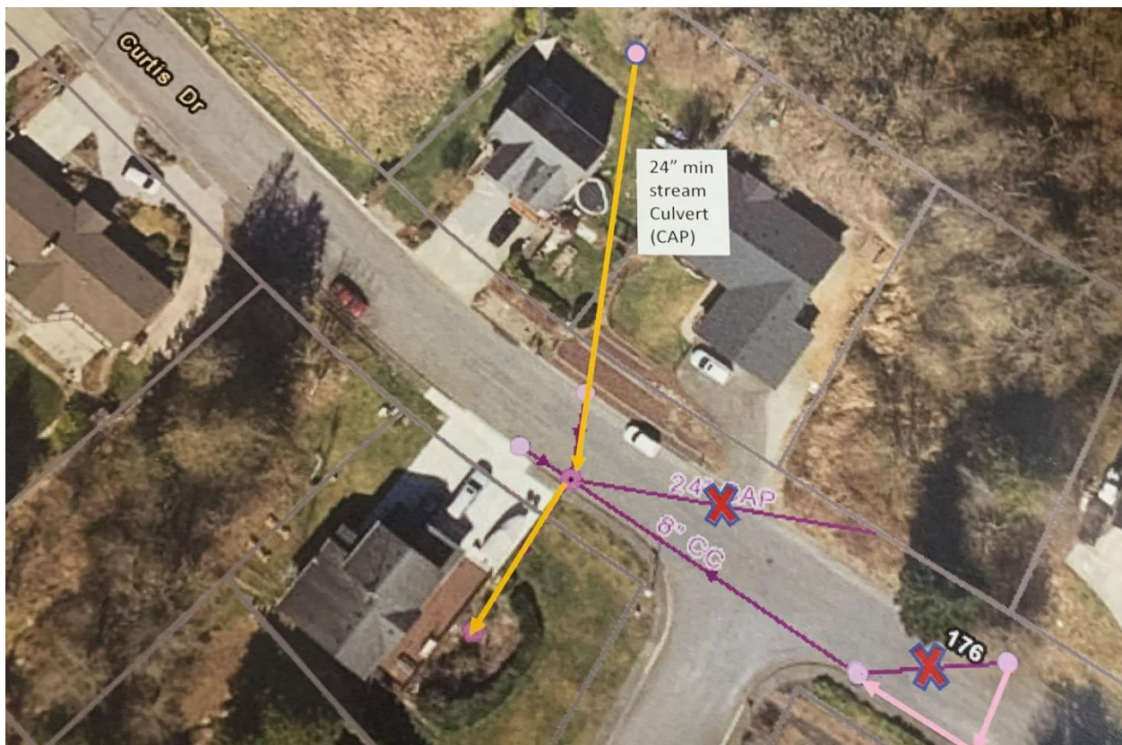
Correcting Stormwater Infrastructure Mapping Information Using Field Surveys and Aerial Imagery
