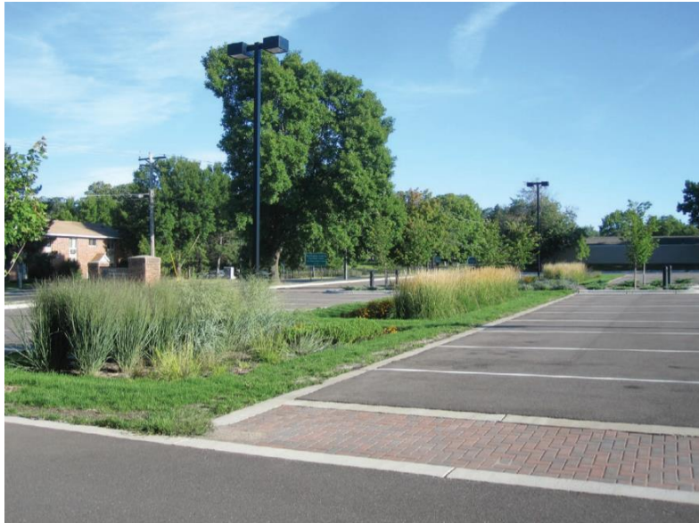
Figure 6-1: Parking lot bioretention (source: US EPA)
