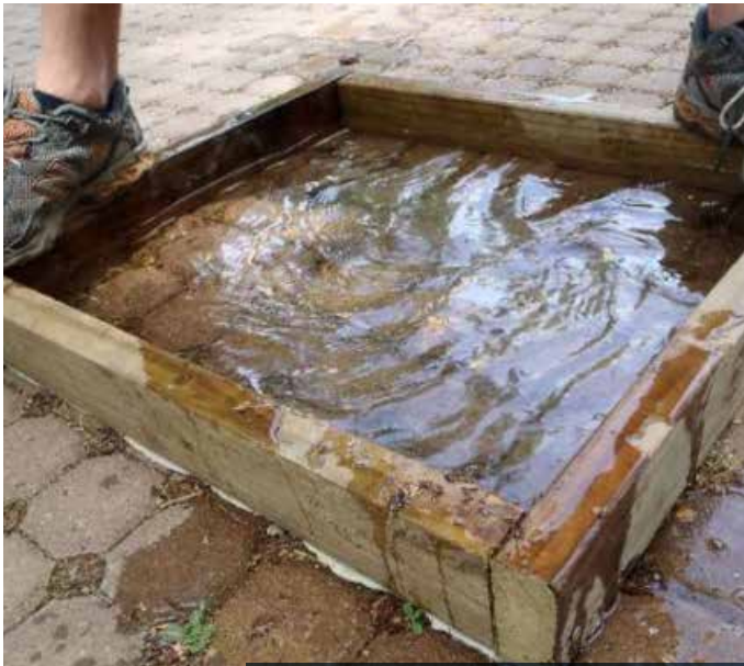
ASTM C1781 test involves measuring the drawdown rate of a section of pavement.
